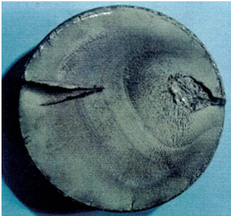
Fatigue Fracture with Beachmarks
